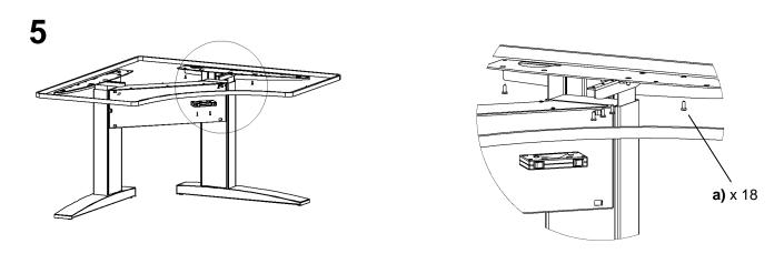
All 18 pcs. screws a) must be tightened for maximum stability.
